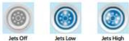
Some devices, like pumps, may have more than one ON state, so the icon will change to reflect the state of the equipment. Below are some examples of 2-speed Pump indicators.
